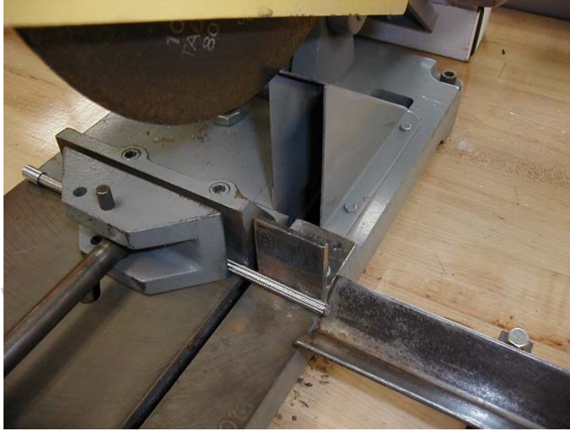
Figure #1: Hose Cut-off – Abrasive Wheel
